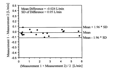
**Figure 4.** Bland-Altman graph showing the agreement between the two series of in vitro measurements at the same location under steady flow conditions: Notice the small mean and standard deviation of the differences between the two series of measurements.
