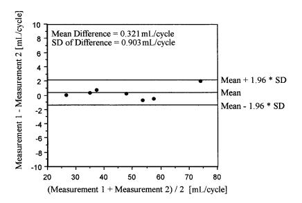
**Figure 6.** Bland-Altman graph showing the agreement between the two series of in vitro measurements at the same location under pulsatile flow conditions: Notice the small mean and standard deviation of the differences between the two series of measurements.
