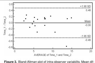
ference between same operator measurements on single data-set is 0.01 cm<sup>3</sup>.
